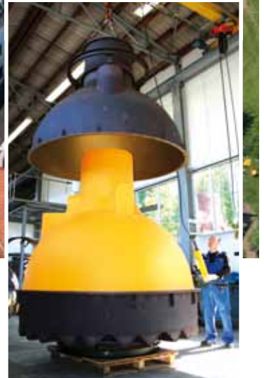
Rainwater storage tank production
